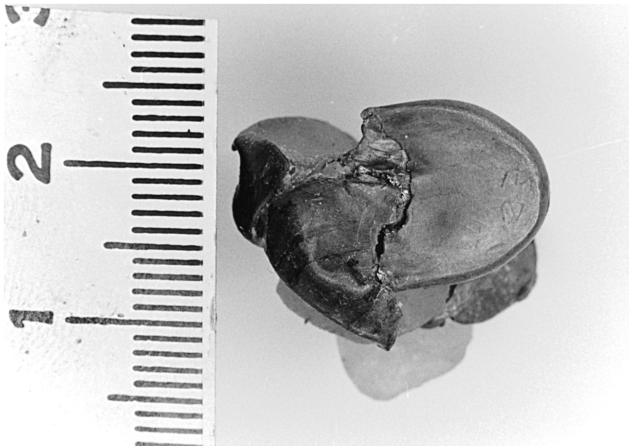
FIG. 5—Physical match of the two 9 × 19 mm FMJ bullet fragments.
