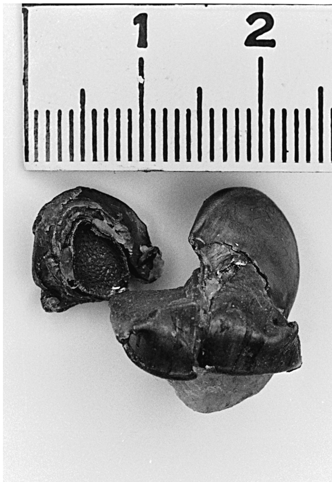
FIG. 6—Physical match of the two 9 × 19 mm FMJ bullet fragments.
